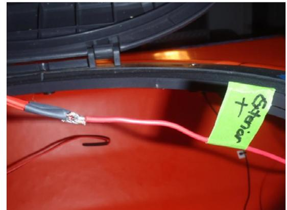
With the exception of the switches, do not make any part of the install permanent until everything is tested. With everything tested and final placement determined, make the final solder connections inside the hull.
